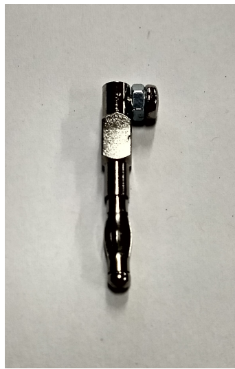
Figure 4.6: Banana plug mechanical fixing for MEMS sensors on vibration generator
